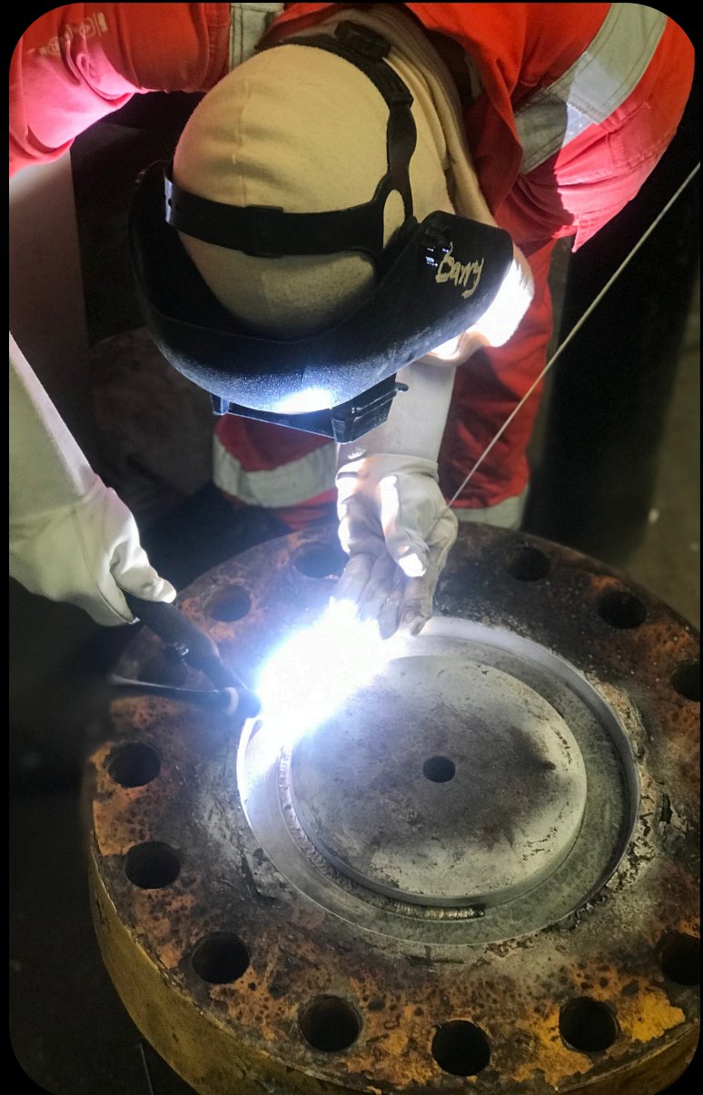
Welding of Drilling Tools and equipment Prior to machining (O-RING)
