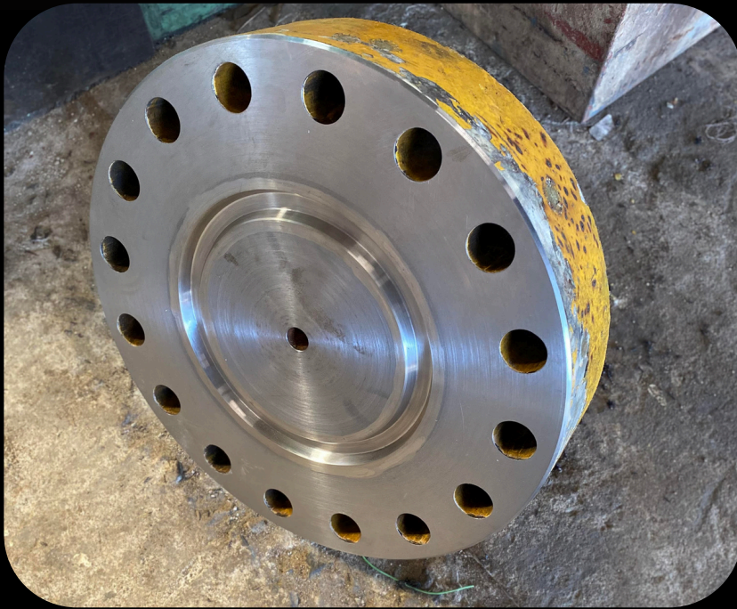
(O-RING) After machining
